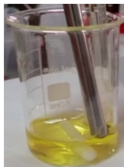
Figure 4 – Methyl Red color (salmon rose) in the borax solution at the titration end point (pH ~ 5) after the addition of 4.8 \text{ mL} of \text{HCl}
